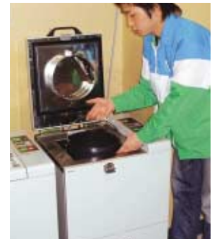
Microwave-type perishable-waste processor
