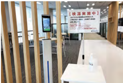
Non-contact temperature measurement system for visitors
