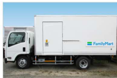
A delivery truck with dual compartments for fixed-temperature food products and chilled food products
