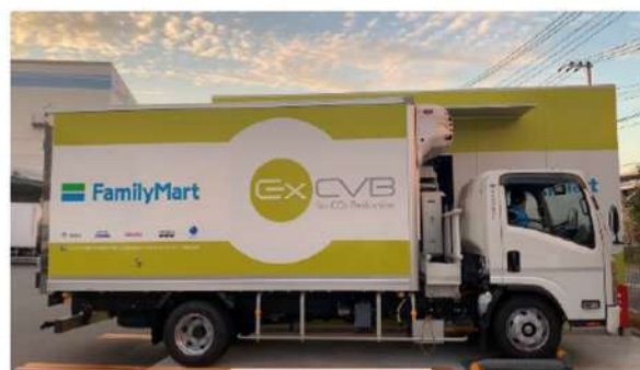
Electric truck with interchangeable batteries
