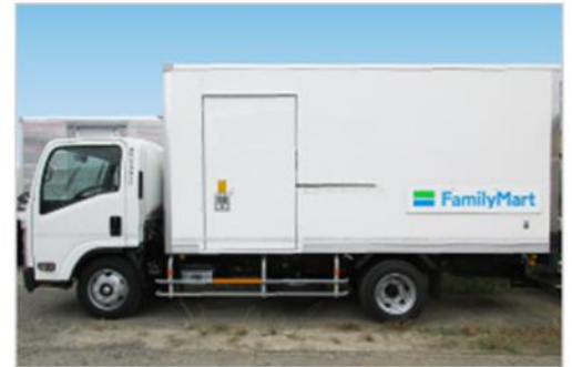
A delivery truck with dual compartments for constant temperature food products and chilled food products
